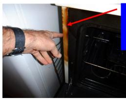
...the oven door gasket is missing resulting is scorched paint...
